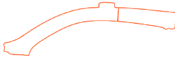
Joining both sub-blanks using laser welding to form the A-pillar blank
