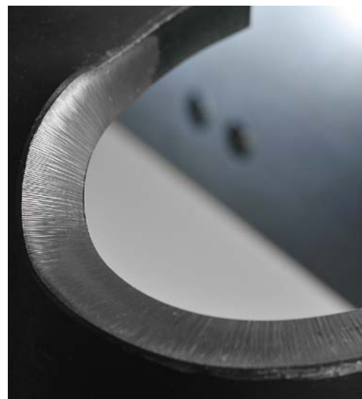
Trailer part made of 12 mm Armstrong® Ultra 700MC, laser cut and bent.
